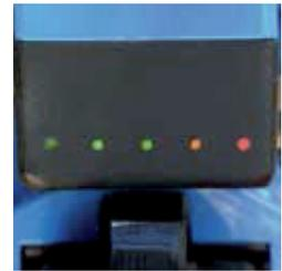
Operate in optimum power range using LED-indicators
